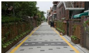
Permeable Pavement (투수성포장)
